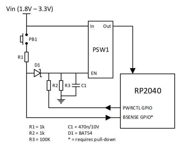
Circuit operation is largely as before, though the BSENSE GPIO now needs a pull-down rather than a pull-up and the GPIO sense is inverted. Note that the PWRCTL GPIO should be floated to turn off rather than pulled low. PSW1 needs to have a suitable low-threshold EN pin; for example, something like Ti TPS22917 should work with Vin down to 1.8V.
