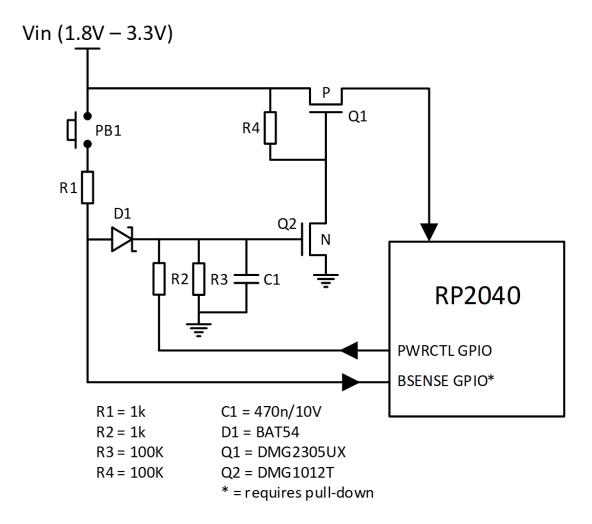
The P and N MOSFETs must have suitably low threshold voltages (the example devices chosen have Vt of 1 volt maximum).
