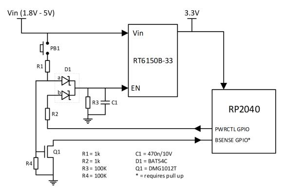
In this example we use the Richtek RT6150B-33 buck-boost SMPS as found on Raspberry Pi Pico, outputting a fixed 3.3V to RP2040.
